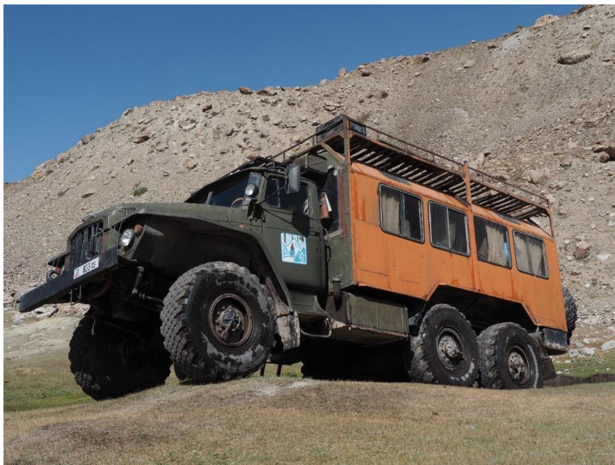
6 Wheel Drive URAL ex-soviet military truck built 1984 aka 'The Beast' (Photo: Andy Stratford)
