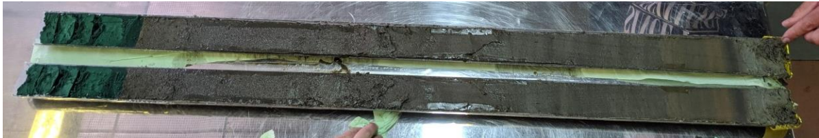
Figure 7: Core extracted from lake Kascadnoe-1. Left is the top (0cm), right is the bottom (109cm). Grey material at the bottom is glacial clay.
