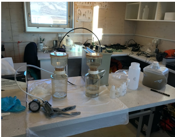
Figure 5: Hand filtration equipment to separate the sediment and dissolved phases of river water. Photo credit Murphy.
