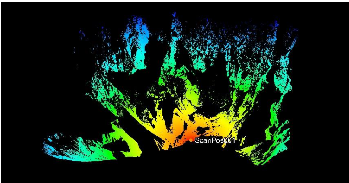
Figure 7. Headwall scan point cloud (18 th October). Point distances range from 1 m (reds), to 2,000 m (blues).
