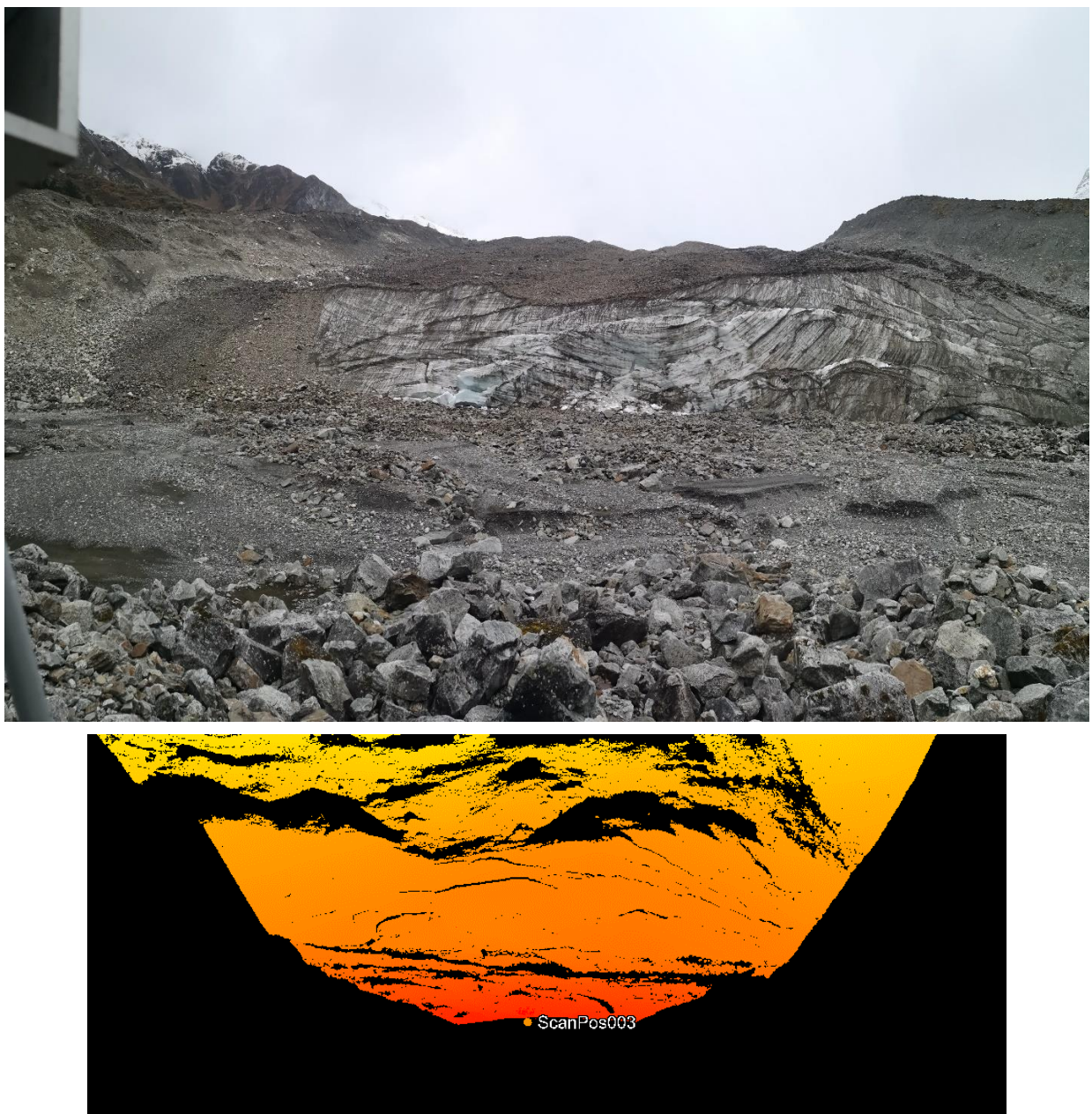
Figure 5. View from the central scan position of the terminal ice cliff and the subsequent point cloud.
