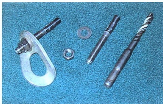
FIG. 25: For bolting we used 8 mm thru-bolts with standard anchor plates.
