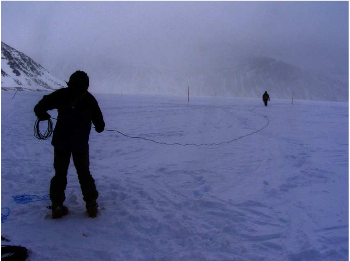
Figure 4.8: Preparation of a radar CMP survey on the glacier - Photo AG, April 2009.
