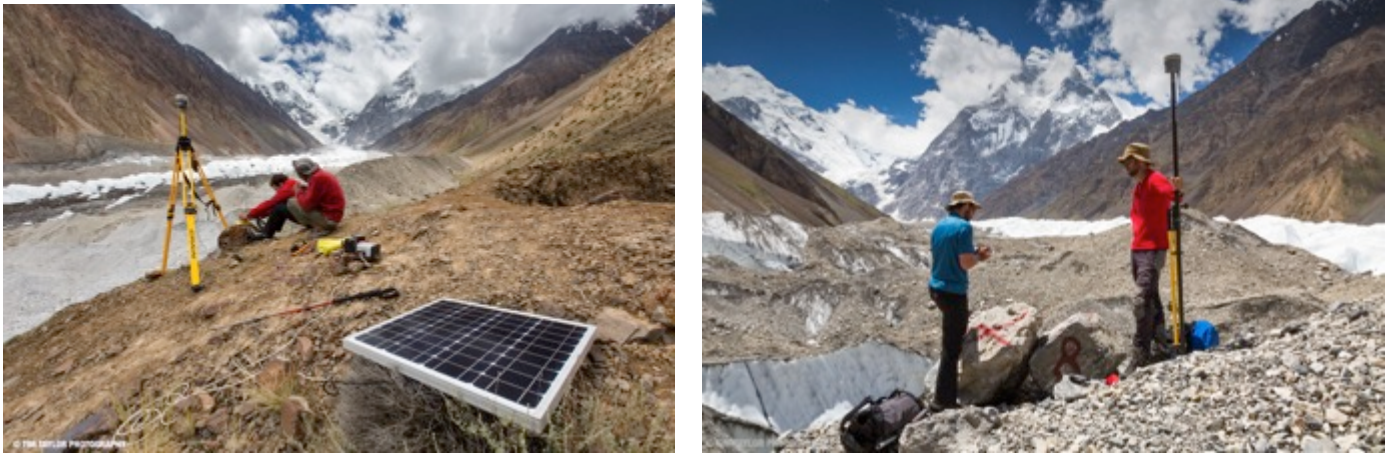
Figure 7. Images showing the base station configuration as seen from the top of Yukshin glacier western lateral moraine (left image) and the rover system on the surface of Yukshin glacier (right image). Copyrights, Tim Taylor, 2015.
