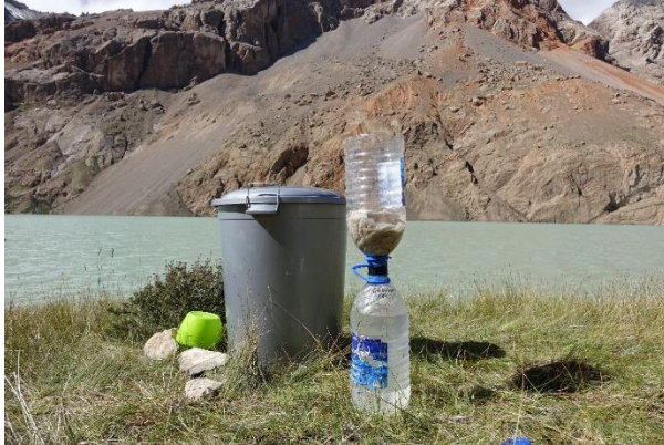
Water was collected from the lake in a in a large settling tank before being filtered and transferred to 10l water bottles.
