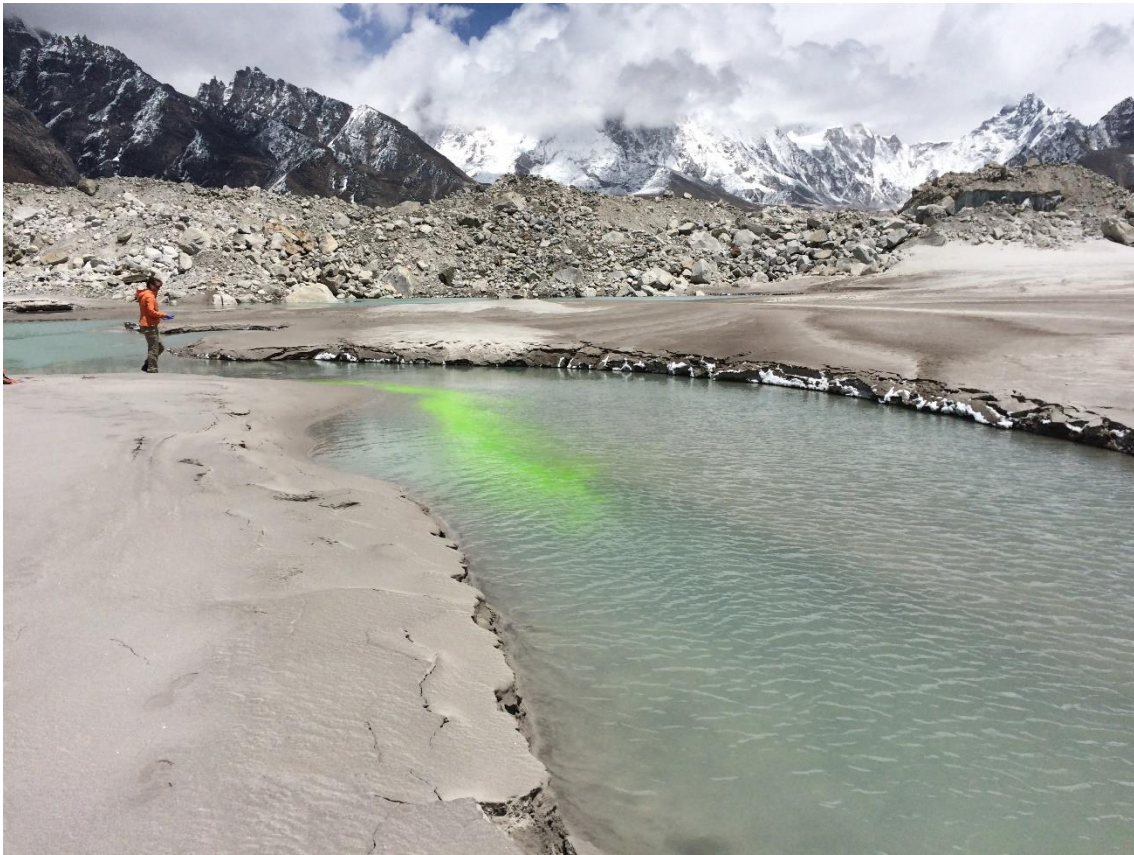
Figure 2: Example dye injection during a dye-test from DIP1, at the terminus of Khumbu Glacier
