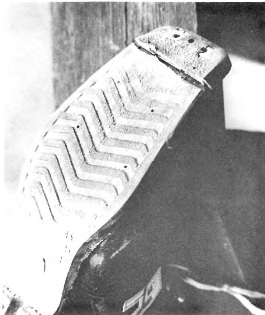
The split across the toe of the boot behind the three pin holes for the binding is clearly visible.
