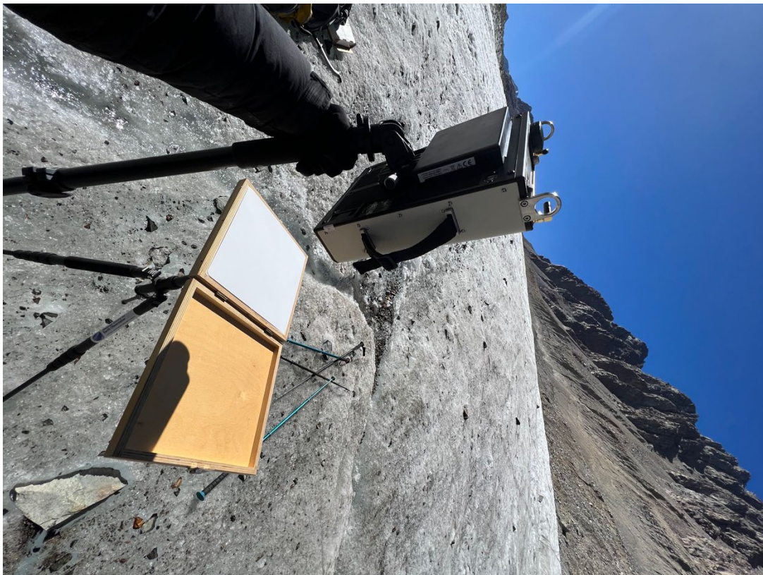
Spectrometer set-up with white standard
