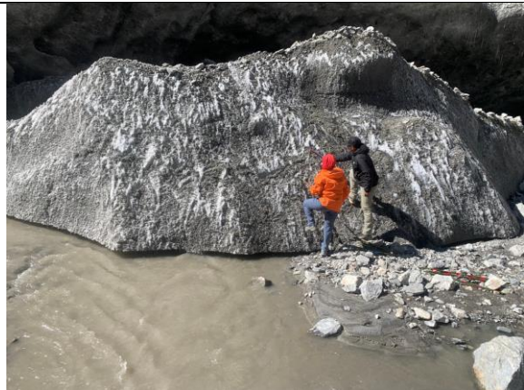
Photo 12. Research assistant (Manisha) and mountain guide (Tula) installing stakes at one of the ice cliff sections.
