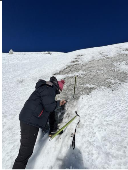
Photo 15. Stake installation and noting GPS points with handheld GPS at Yala Glacier's ice cliff and
