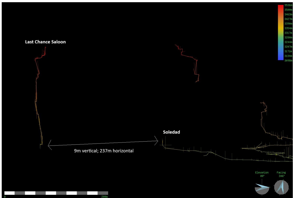
Figure 32. Survev data centre-line showing that the undescended pitch at the bottom of last Chance Saloon Pot (left) is 237 m laterally and 9 m lower than the top of the boulder choke at the upstream end of the Pisco and Codeine Streamway in Tragadero de la Soledad. This is by far the largest of the two streamways in Tragadero de la Soledad, and it must drain a large area including surface sinks.
